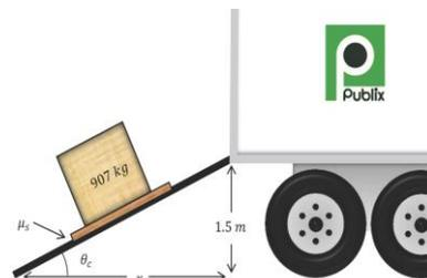
**Figure 9.** Unloading a Publix supply truck by sliding a pallet down a ramp [80].
