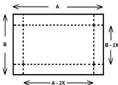
**Figure 13.** Constructing an open topped box (raft) from a flat sheet
