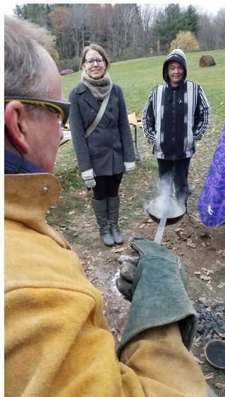
ABOVE LEFT: Fergus Milton holds a clay ball that he has just extracted from the furnace. He lets it cool before breaking it open to reveal the newly formed copper inside. (Taken by Dr. Timothy Messner)
