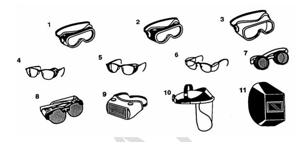
Eye and face protectors are identified below by number and type. Refer to Table 1 for recommended usage applications.
